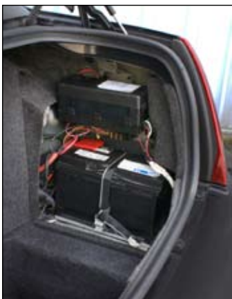
The battery and power distribution center have been relocated inside the trunk on the passenger side.
